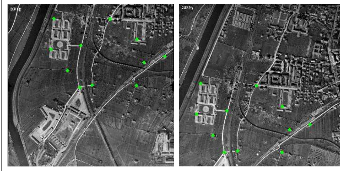
Figure 3: Automated search of GCPs by cross-correlation in a user-defined search region ( i.coregister )
